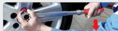
4. ADJUST and START tightening (prescribed torque direction) 5. when you hear audio signal (click), the designated torque is reached - STOP TIGHTENING!
