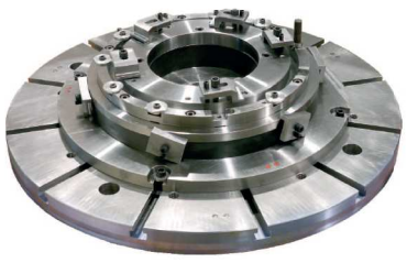
FIXTURE FOR LATHE
